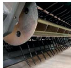
Pick-up blade, pick-up roller with spring tines
