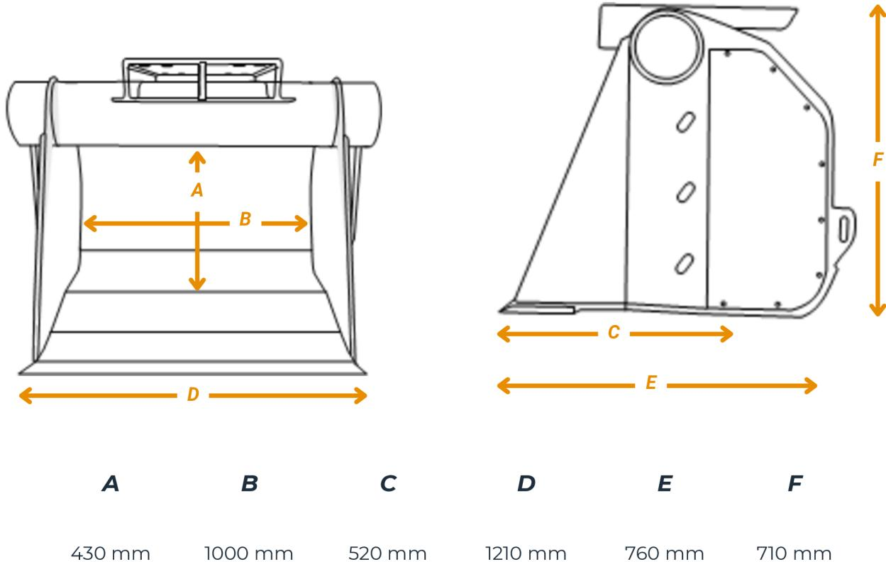
**Please Note:** The given weight is for a bucket fitted with a 20 mm fragment kit. The weight may vary depending on the fragment size selected. The compatible carrier weight range may change if the screening bucket is used in conjunction with a tiltrotator.
