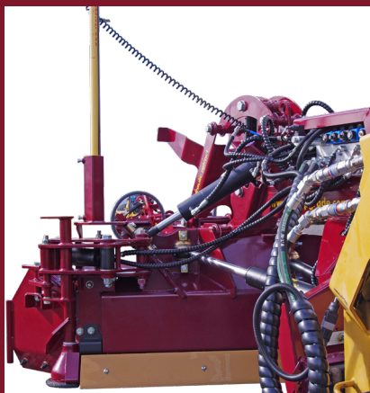
Pivoting rear blade to precision grade in reverse
