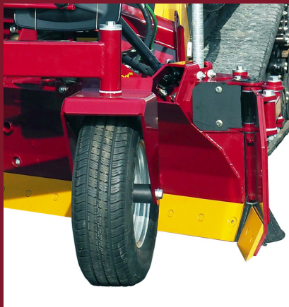
Hydraulic wings control material in both directions
