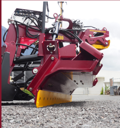
Up to 36° pitch forward to finish grade in six-way mode
