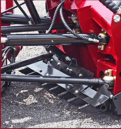
No grease - all linkages are sealed for life. Optional Scarifiers
